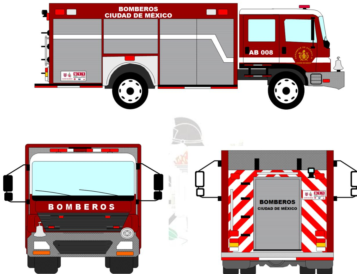
IMAGEN 2 OPCION CHASIS/CABINA COE (cab over engine).
